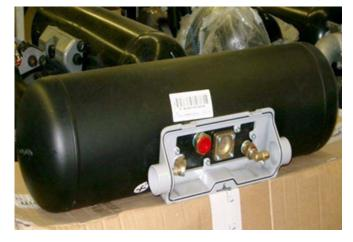
**Diagram #2** Incorrect tank storage and orientation.
